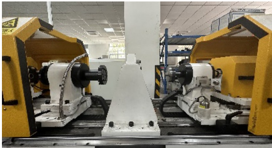
图11 谐波齿轮减速器试验台 Fig. 11 Test bench for harmonic gear reducers
